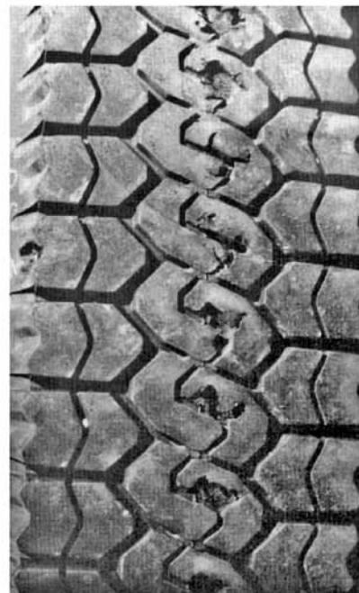
Example of Dyno Damage
