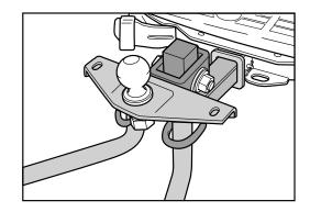
Clamp-On Bumper Hitch – As the name suggests, this type of temporary hitch clamps onto the bumper assembly. Nissan does not recommend the use of this type hitch for a number of reasons. It may interfere with performance of the energy-absorbing bumper. And because the bumper was not designed to carry this type of load, it could damage the bumper and bodywork, and may possibly result in trailer separation during towing. Therefore, tow only with a permanent hitch.
