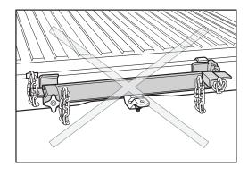
5th Wheel or Gooseneck Hitch – Mounted in the bed of a pick-up and designed for heavy-duty applications, these types of hitches are not available from Nissan but can be purchased from a professional supplier of towing equipment.\*
