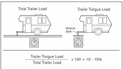
weight, within the limits of the maximum trailer tongue load allowable. For example, to determine the proper trailer tongue load for a 1,500-lb. trailer, multiply the weight of 1,500 lbs. by 10% to arrive at a figure of 150 lbs.
