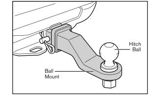
in a number of weight capacities and sizes. Therefore, always make sure the hitch ball selected has the proper shank diameter and weight rating for the ball mount as well as the coupler on your trailer. Using a 1<sup>7</sup>/<sub>8</sub>" hitch ball in a 2" coupler, for example, could result in the
