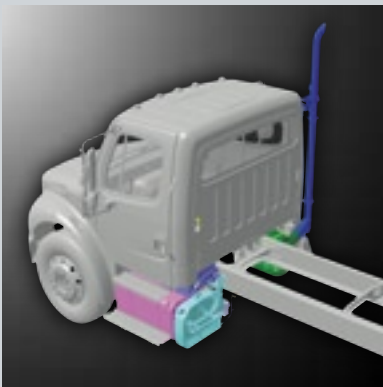
CLEAR BACK OF CAB TAILPIPE Clear left-hand and right-hand transmission PTO mounting locations
