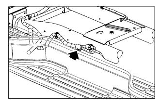
For vehicles not equipped with heavy duty trailering, the harness is clipped to the vehicle's frame behind the spare tire mount. The harness requires the installation of a trailer connector, which is available through your dealer.
