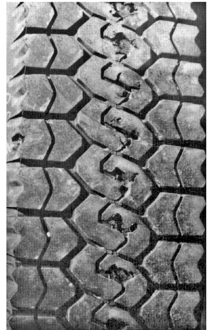
Example of Dyno Damage
