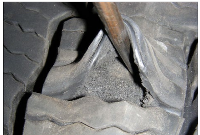
EFFECT: Internal Deterioration of the Tread Rubber CAUSE: Prolonged Use of Dynamometer
