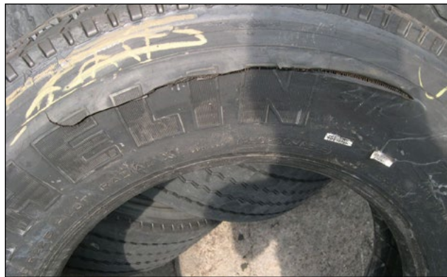
Fatigue Rupture or “Zipper”
