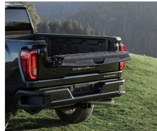
INNER GATE WITH WORK SURFACE The opened inner gate provides a work surface as well as second-tier loading.
