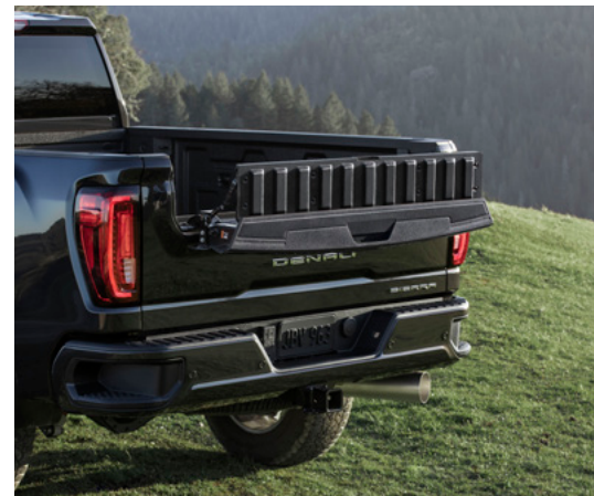
INNER GATE LOAD STOP The inner gate also includes a load stop to help prevent second-tier items from sliding out of the bed.
